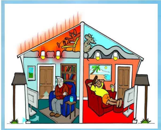
Energy saving by using Loft Covers over downlights
